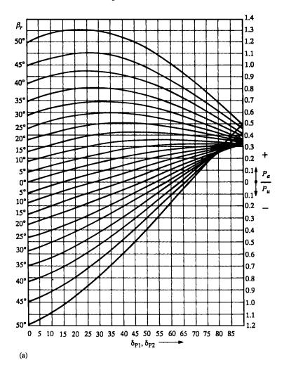
Figure 5.8(a-c) Axial thrust,  $P_a$ , relative to  $P_u$  for (a)  $17\frac{1}{2}^{\circ}$ , (b)  $20^{\circ}$  and (c)  $22\frac{1}{2}^{\circ}$  pressure angles, applicable to all angles of the shafts
