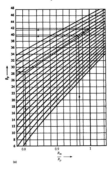
Figure 6.3(a,b) N-gear spiral angle
