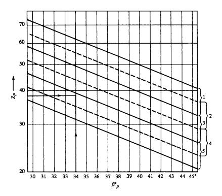
Figure 6.2 Standard cutters (En) – selection of blades ( $Z_P = \text{no.}$  of teeth – crown gear, calculation 5, page 118;  $\beta_P = \text{spiral}$  angle, calculation 15, page 122)
