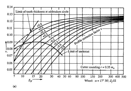
Figure 5.9(a,b) Tooth profile factor, y (to be inserted into the Lewis formula) for increased cutter roundings
