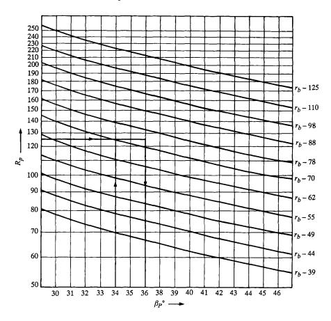
Figure 6.4 Selection of En cutters ( $\beta_p$ =spiral angle;  $R_p$ =reference cone distance) Example:  $\beta_p$ =36°;  $R_p$ =125 mm. Cutters En 5-70 will be used. The resultant spiral angle = 34°
