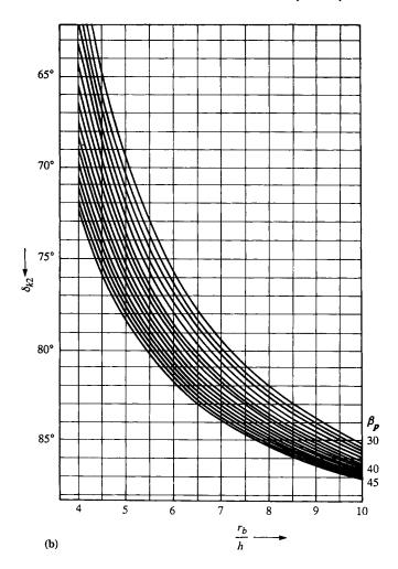
At the intersection with the corresponding curve of the angle  $\beta_p \times r_b$  (spiral angle  $\times$  cutter) designation, results from the cutter and h are found in the same manner. This is carried out in Figures 6.6(a), 6.6(b) and 6.6(c), giving the following tilt angles:  $C = 0^{\circ}$ ,  $C = 1^{\circ}30'$  and  $C = 3^{\circ}$ .
