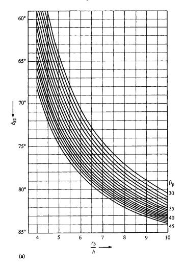
Figure 6.6(a-c) Graphs for cutter spindle tilt: (a)  $C = 0^{\circ}$ ; (b)  $C = 1^{\circ}30'$ ; (c)  $C = 3^{\circ}$
