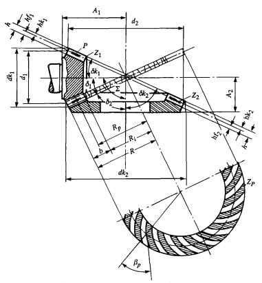
Figure 6.1 Oerlikon spiral bevel gear dimensional layout
