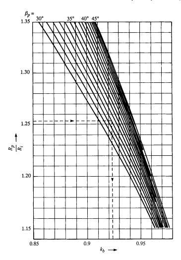
Figure 6.5 Standard cutters (En) – calculation factor  $k_b$  ( $R_i$ =inner cone distance;  $R_p$ =reference cone distance:  $m_{ni}$ =normale module;  $m_p$ =normal module)
