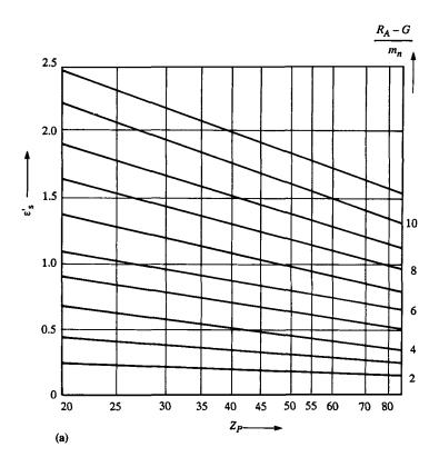
Figure 5.6 Spiral overlap and profile overlap:
