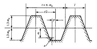
Now the tooth profile can be laid out, and the involute curves between the addendum,  $d_{kn1}$ , and base circle,  $g_{gn1}$ , can be generated in the known way through the terminal points of the normal thickness of tooth,  $S_n$ , plotted on the pitch circle,  $d_{gn1}$ .
