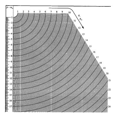
Figure 5.2(a) Graph for checking the position of the gear hob—see also Figures 5.2(b) and 5.2(c). If the positions of gear hobs are to be checked which have a cone distance  $R_A$  not given in the graph above, then the positions must be found by drawing them out on millimetre graph paper (Figures 5.2(a), (b) and (c) should be enlarged to 200% their present size for accurate measurement in mm)
